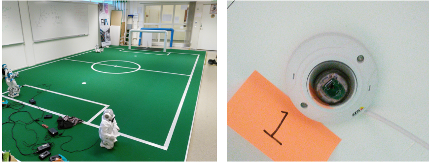
Figure 6.1: Humanoid lab (left) equipped with four ceiling cameras (right).
