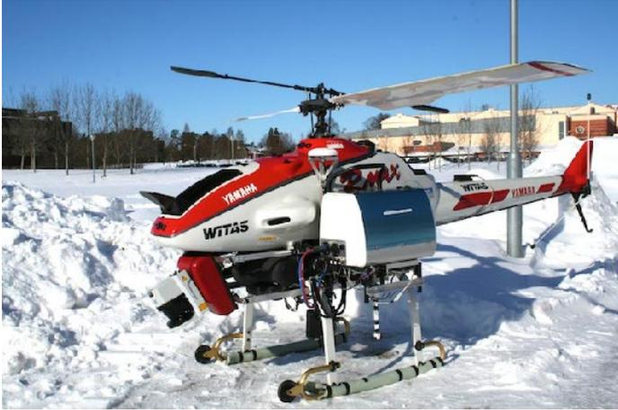
Figure 2.2: The Yamaha RMAX helicopter with a laser range finder mounted on a rotation mechanism.
