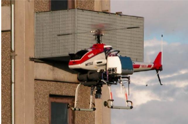
Figure 1.1: The UASTechLab RMAX helicopter platform.
