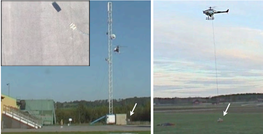
Figure 2.17: Two frames of video presenting the prototype mechanism for carrying and releasing packages using an electromagnet. An arrow points to a package being carried. The top left picture presents the on-board camera view.
