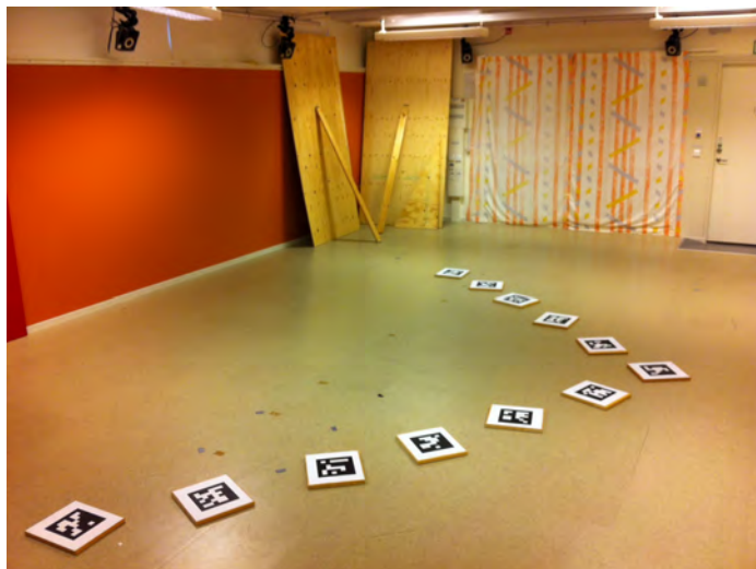
Figure 3.31: The marker setup used for evaluating the accuracy of the map building method. Vicam cameras of the reference system visible at the top of the image.
