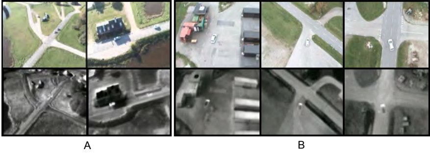
Figure 2.20: A. Two frames from video sequence with the UAV hovering close to a road segment observing two cars performing overtaking maneuver. B. Three frames from video sequence with the UAV following a driving car passing road crossings. Top row contains color images and bottom row contains corresponding thermal images.
