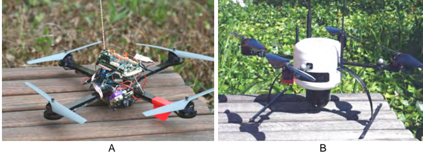
Figure 3.4: The Hummingbird quadrotor UAV with the LinkBoard I flight control board, B. The LinkQuad quadrotor UAV platform.
