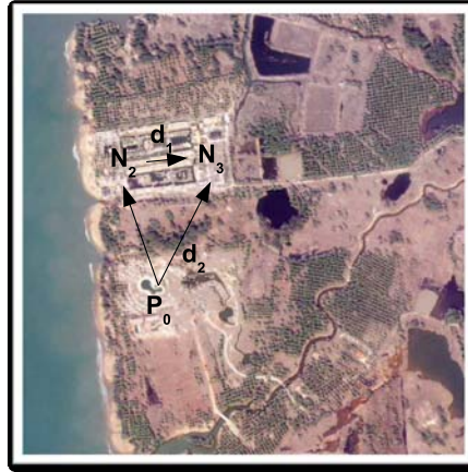
Figure 7.15: Provided that P_0 is assigned to N_3 , the distance P_0 has to move to reach N_3 depends on P_0 's previous commitments. If P_0 is allocated to N_2 , there is one distance ( d_1 ) for P_0 when the platform is also allocated to N_3 . If N_3 is platform P_0 's first allocation, the distance is counted from the platform's start position instead ( d_2 ). The distance constraints describe such distance rules for all possible platforms and task combinations.
