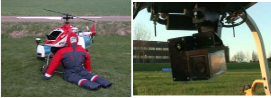
Figure 6.3: The UASTech UAV and the onboard camera system mounted on a pan-tilt unit.
