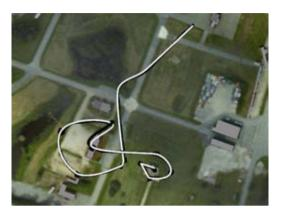
Figure 8.3: Autonomous survey mission to two buildings, which are photographed from each side.
