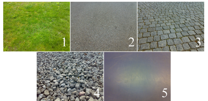
Fig. 1: Terrain types that are detected by the presented system: 1. Grass. 2. Asphalt. 3. Gravel. 4. Pavement. 5. Indoor Floor.
