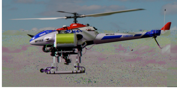
Figure 2. The UASTech Yamaha RMAX helicopter system [27,28].
