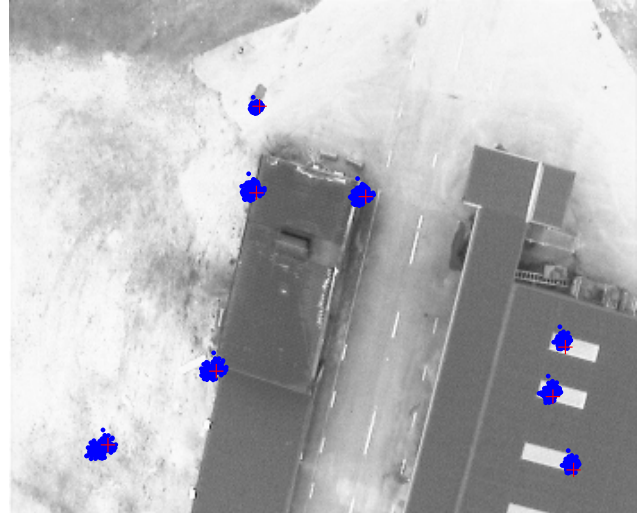
Figure 2. The scenario seen from the on-board vision sensor, together with particle clouds representing the landmarks/map features.
