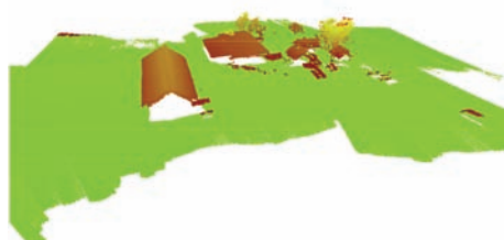
(a) Surface model generated from the lidar system.
