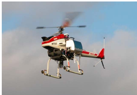
Fig. 2. The WITAS RMAX autonomous helicopter.
