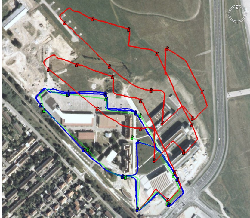
Figure 12. Result from applying RFID-SLAM outdoors while driving with 1.58m/s for more than 2.5km with a Zerg robot. Trajectories are visualized by GoogleEarth, showing the odometry trajectory (red), the ground truth trajectory (blue), and the corrected RFID trajectory (green). Whereas the odometry strongly diverges from the driven path, the corrected trajectory is close to the ground truth.
