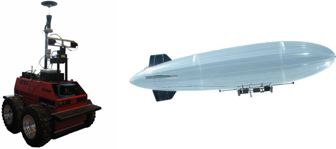
Figure 1: The ATRV rover Dala and the 10m long blimp Karma. Both robots are equipped with a stereovision bench.
