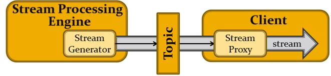
Fig. 5. Realizing a stream using a topic.
