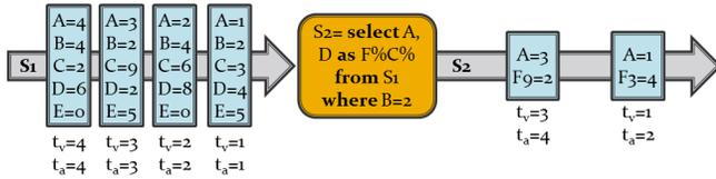
Fig. 2. Stream processing example: select
