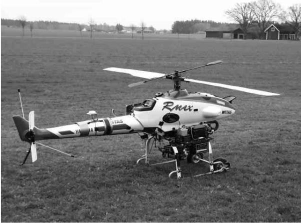
*Figure 1: The WITAS UAV Platform*
