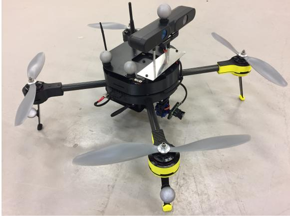
Figure 7: LinkQuad platform with an Asus Xtion PRO depth camera.
