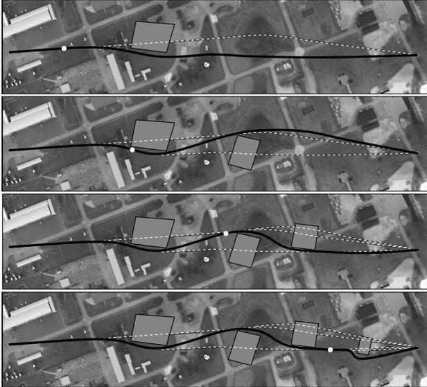
**Figure 1. Paths generated during the experimental flight. Solid black line - updated path; white dot - helicopter position; white dashed line - invalid path; polygon box - forbidden region.**
