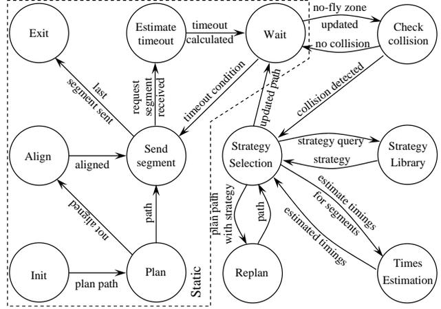
**Figure 9. The dynamic path replanning automaton**
