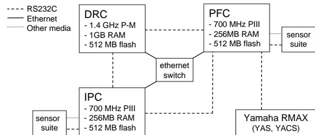
**Figure 3. On-Board Hardware Schematic**
