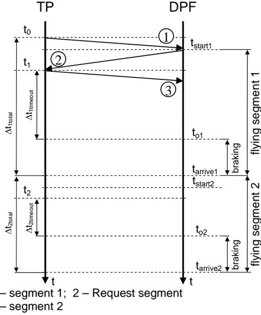
**Figure 8. Execution timeline for trajectory consisted of 2 segments**
