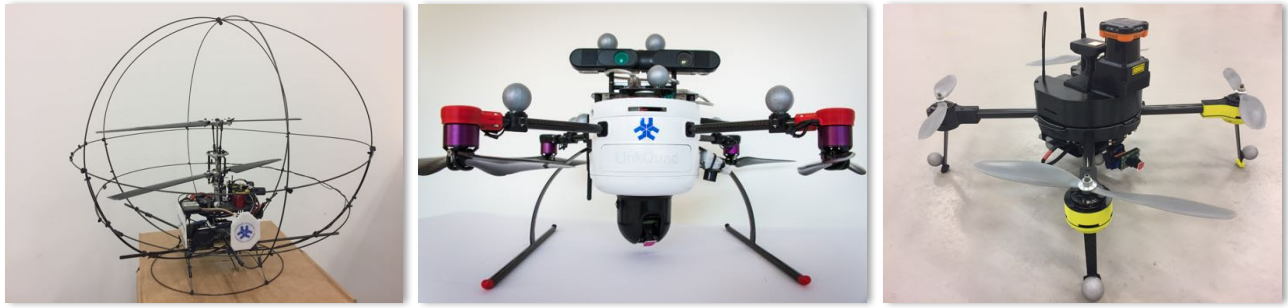
Fig. 7. The LinkMAV coaxial platform (left). The LinkQuad platform with a structured-light 3D scanner and a Pan-Tilt color camera unit (middle). The newest generation of the LinkQuad platform with a laser range finder, an external GPS and a Pan-Tilt-Roll color camera unit (right).
