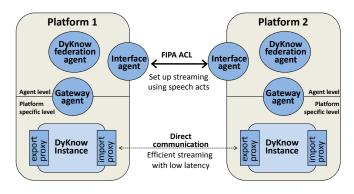
Figure 3. An overview of the components of a DyKnow Federation.
