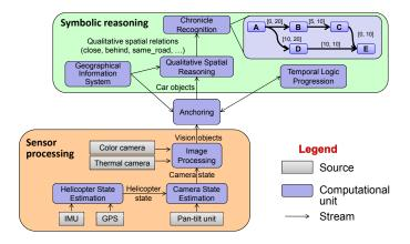
Figure 1. An overview of how the incremental processing required for a traffic surveillance task could be organized.
