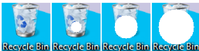
Figure 3.5: Example of how obstruction affects a image for the values 0, 25, 50, 75 respectively
