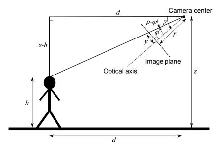
Fig. 3: To estimate the ground distance d between the UAV and the person, we assume a horizontal ground plane and a person height h. The angle  $\varphi$  is obtained from normalized image coordinate y of the upper edge of the bounding box and the effective focal length f. The UAV altitude z and camera pitch  $\rho$  are known. The distance is obtained using simple geometry by considering the larger triangle in the figure.
