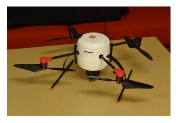
Fig. 1: LinkQuad platform with the color camera sensor module.
