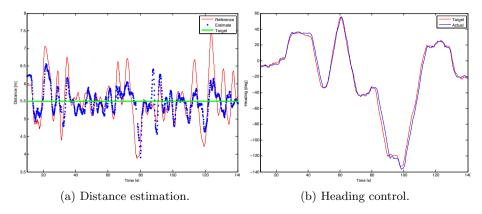
Fig. 5: The estimated relative distance of the target relative to UAV (a), target and actual heading (b) during the leashing experiment.
