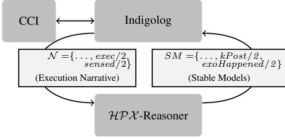
**Figure 3.** Information flow between Indigolog and the ASP-based  $\mathcal{HPCX}$  reasoner
