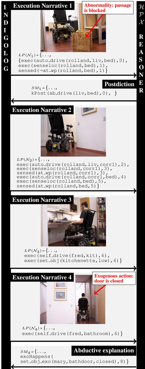
Figure 5. Communication between Indigolog and  $HPX$ -reasoner during the scenario
