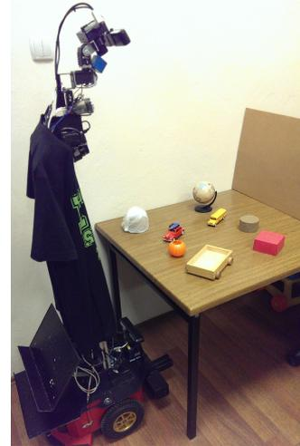
Figure 6. Pioneer 3-DX and the objects used in the tabletop exp.
