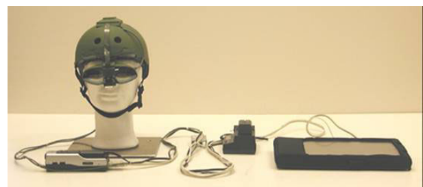
Figure 4: A video see through MR system (Gustafsson et al 2005)
