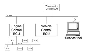
Figure 1. An heterogeneous automotive control system
