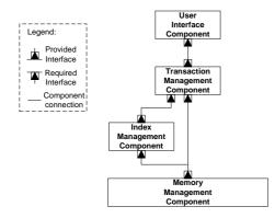
Figure 3. The basic architecture of COMET
