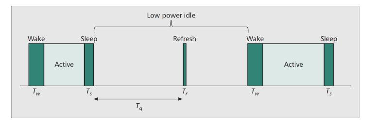
$T_s$ : Time to low power idle (sleep)  $T_w$ : Time to go to active (wake)  $T_q$ : Interval without signalling  $T_r$ : Refresh signalling interval
