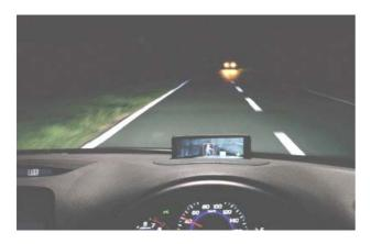
Fig. 1. NVS provide an enhanced view of the road ahead. The example shows Honda's intelligent NVS, which has detected a pedestrian. The system warns the driver by highlighting the pedestrian on the head-up display and by blinking an icon and sounding an alarm (more information can be obtained from Honda's web-site, [10])
