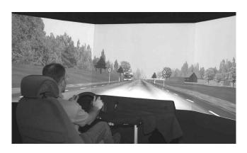
Fig. 3. The fixed-base driving simulator used in our study is softwareoriented and allows for rapid prototyping of new driver assistance systems and HMI-features.
