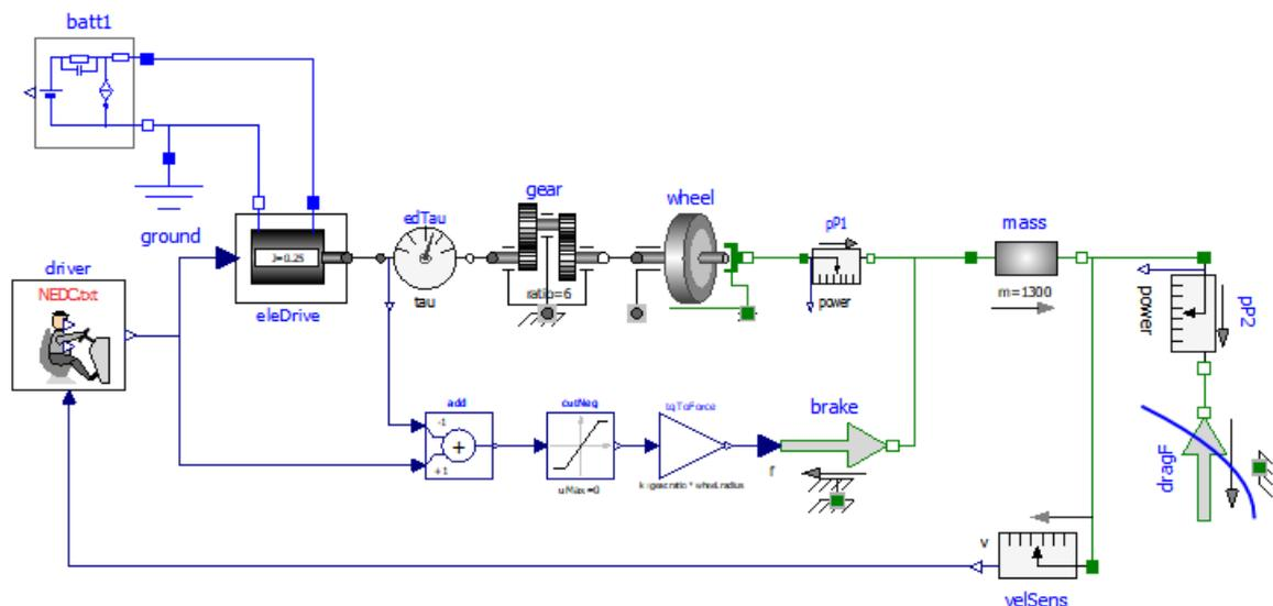
A model library in Modelica with model components relevant for electric cars will be made available. Tool support for modeling, simulation, requirement formalization, requirement verification, optimization, etc. will be available using OpenModelica.
