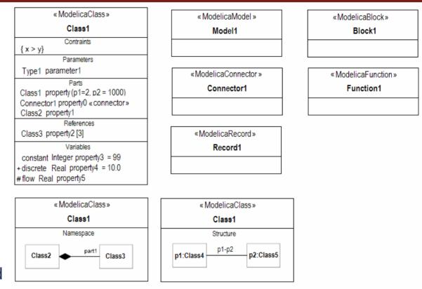
Class Diagram defines Modelica classes and relationships between classes, like generalizations, association and dependencies ModelicaML - Internal Class Diagram
