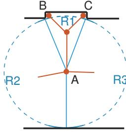
**Figure 5.** Region  $R1$  of vertex  $A$  is caused by a small niche in a wall. Since  $A$  lies in a large area the distance along the GVD from  $A$  to the corner vertices  $B$  and  $C$  is rather big. However, most part of the connection to these vertices lies within the maximal inscribed circle and will thus be subtracted during the RSM computation resulting in a small RSM value for region  $R1$ .
