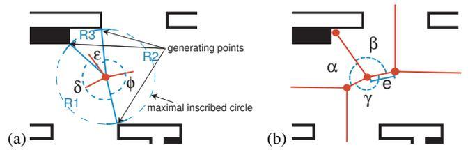
**Figure 2.** Different kinds of annotations to the GVG-based route graph: (a) Vertex signature containing the distance of the generating points (radius of the maximal inscribed circle) and angles between the connections to the generating points, (b) relative position information given by the angles between departing edges and the length of the edges.
