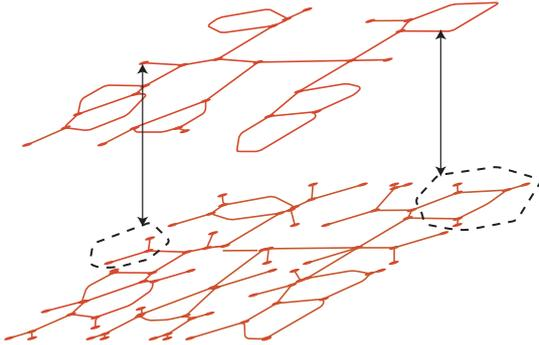
**Figure 7.** A two-layer hierarchical route graph representation with the original GVG at the bottom and a coarser route graph layer on top of it. Two examples of how parts of the detailed level are represented by a vertex or an edge of the coarser level are shown by the arrows.
