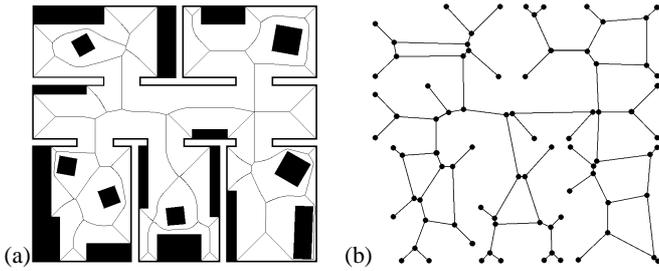
**Figure 1.** (a) The generalized Voronoi diagram (GVD) (fine lines) of a 2D environment, (b) the corresponding generalized Voronoi graph (GVG) with vertices placed at the position of the corresponding meet points for visualization.
