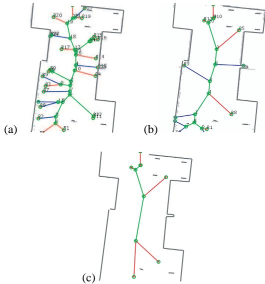
**Figure 9.** Simulation of different sensor properties: (a) shows the GVG of a robot with high and (b) of one with low sensor noise. Identical coarse route graphs are computed from both GVGs (c).
