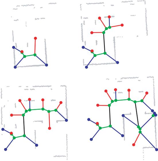
**Figure 3.** A sequence of growing global GVGs (starting with the local GVG of the robot’s start position) constructed during the exploration of an unknown environment.
