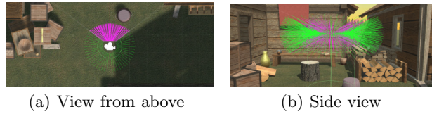
Fig. 12. Third-person example of 360 peripheral: forward-facing rays (magenta), backward-facing rays (green).
