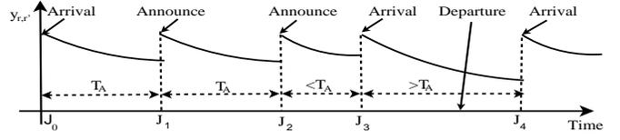
Fig. 2. Jump times and renewal periods in the renewal process for *RMT*. At  $J_0$  peer 1 arrives, at  $J_1$  peer 1 performs an announce, at  $J_2$  peer 1 performs another announce, at  $J_3$  peer 2 arrives and at  $J_4$  peer 3 arrives. Peer 2 departs some time before  $J_4$ .
