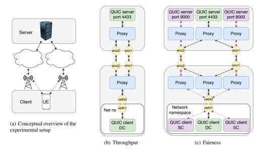
Figure 2: Testbed for throughput and fairness tests.
