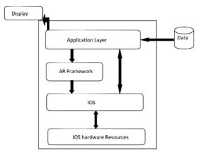
Figure 11. The software architecture of Minnesmark
