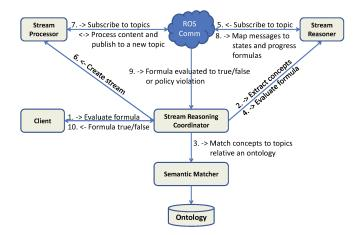
Fig. 5: The stream reasoning architecture.
