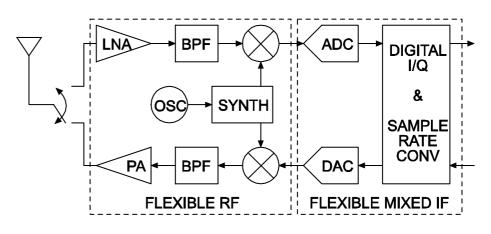
Figure 2. Digital-IF transceiver with flexible RF and mixed-signal
