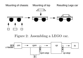
Figure 3: The first half of the LEGO car factory.
