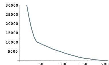
It starts at an altitude of 59404 (not shown in the diagram) at time zero, gradually reducing it until touchdown at the lunar surface when the altitude is zero
