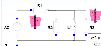
A more specialized class TemperatureElectricalCircuit is created by changing the types of R1, R3, to TempResistor
