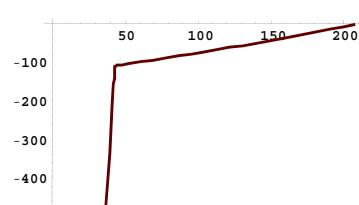
The rocket initially has a high negative velocity when approaching the lunar surface. This is reduced to zero at touchdown, giving a smooth landing
