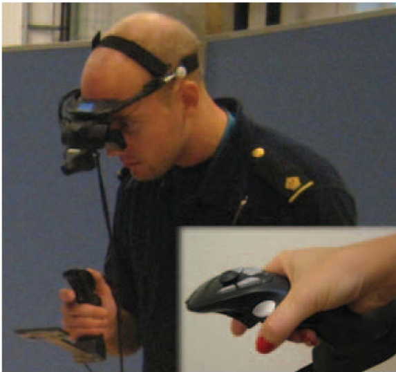
Fig. 1. The redesigned interaction device, which allows the user to choose a virtual object and place it on the digital map.
