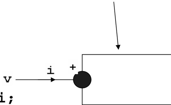
Keyword **flow** indicates that currents of connected pins sums to zero.
