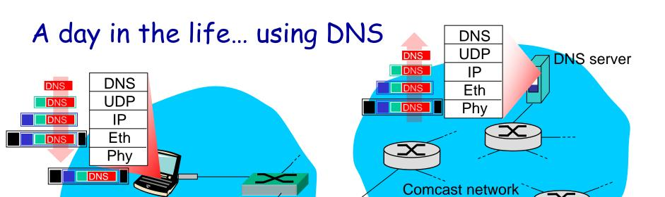
❖ IP datagram containing DNS query forwarded via LAN switch from client to 1<sup>st</sup> hop router
