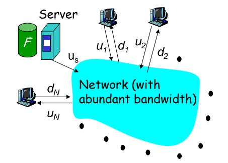
Time to distribute F to Nclients using client/server approach = d<sub>cs</sub> = max { NF/u<sub>s</sub>, F/min(d<sub>i</sub>) } i increases linearly in N (for large N)
