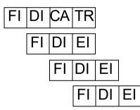
The compiler reorganises the code and tries to find an instruction that does not depend on the loaded value and that can be placed after the LOAD:
