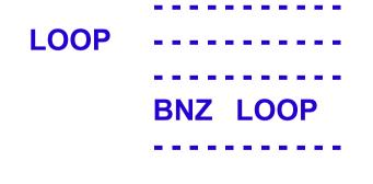
After the loop has been executed for the first time and left, it will be remembered that BNZ has not been taken. Now, when the loop is executed again, after the first iteration there will be a false prediction; following predictions are OK until the last iteration, when there will be <u>a second false prediction</u>.
