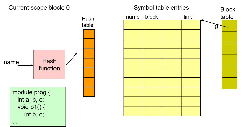
insert p1 and enter a new scope block (2)
