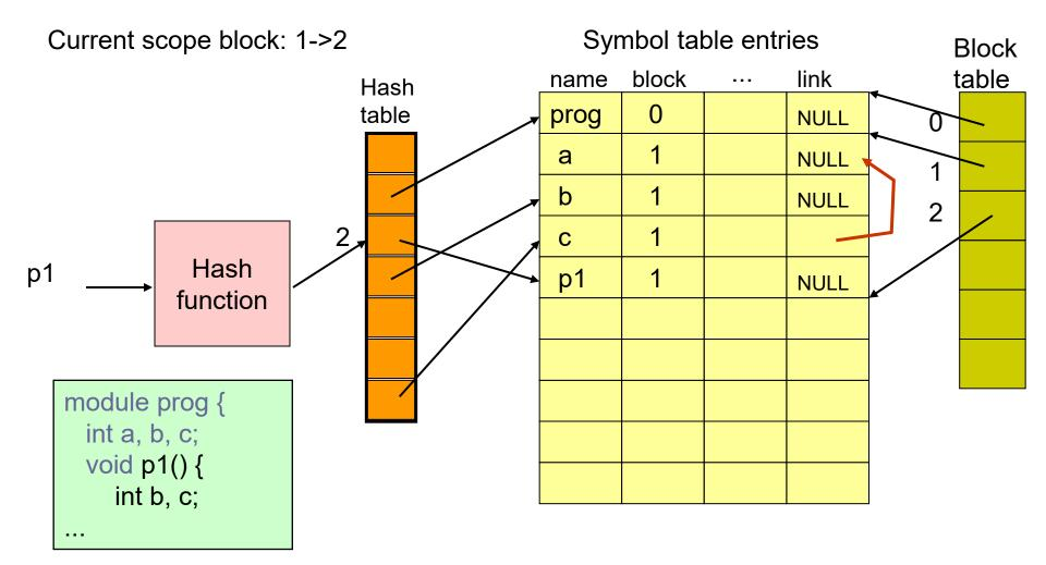
insert p1 and enter a new scope block (2)
