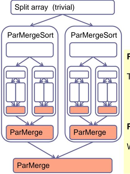
NB: ParMerge (time logarithmic in input size) does all the heavy lifting work in ParMergeSort
