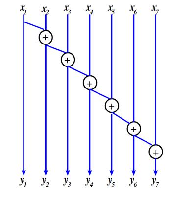
Task dependence graph: linear chain of dependences  $\rightarrow$  seems to be inherently sequential — how to parallelize?
