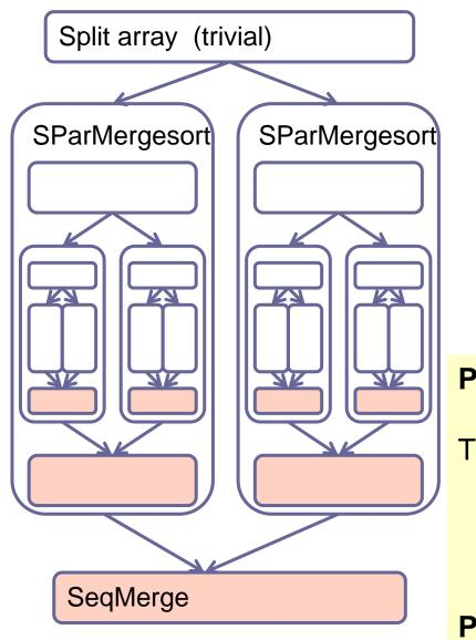
NB: SeqMerging (linear in input size) does all the heavy work in Mergesort
