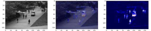
Figure 7: Heatmap of pixelwise \mathcal{L}_1 loss in image containing anomaly. Model parameters: (Ratio: No, L1 Size: 256, LR: 10^{-4} , Latent Size: 64)
