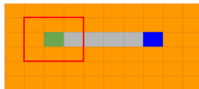
Figure 5: The green square is the agents current position, the blue square is the goal position and the gray squares is the path between the start and the goal. The red line indicates the input states received by the agent.
