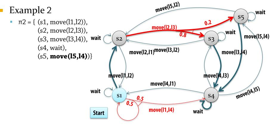
•  $h_1 = \langle s1, s2, s3, s4, s4, ... \rangle$   $P(h_1 \mid \pi_2) = 1 \times 1 \times 0.8 \times 1 \times ... = 0.8$
